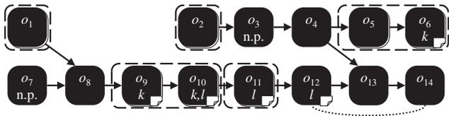
Fig. 4. Parallel region formation example. Operator instances labeled “n.p.” are not parallelizable (e.g., due to unknown state). The letters  $k$  and  $l$  indicate key attributes. The dotted line from  $o_{12}$  to  $o_{14}$  indicates a fusion dependency. Dashed ovals indicate unexpanded parallel regions. The paper icons indicate stateful operators.
