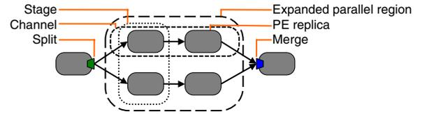
Fig. 3. Stream graph, from the runtime's perspective.
