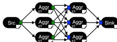
Fig. 8. Expanded stream graph for a two-way shuffle.
