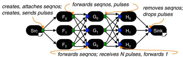
Fig. 6. Splitter and merger responsibilities in a shuffle.
